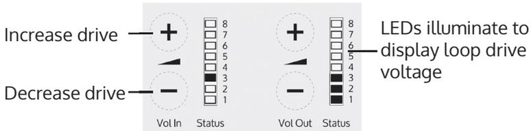
If the amplifier does not have a loop attached, turn off the red loop fault LED 8 by adjusting the drive down to off.
