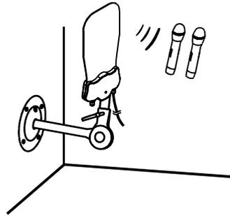
Fig. 3: Wall-mounted to an optional MS-90 wall bracket
