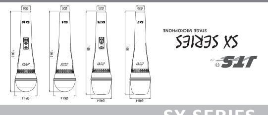
The SX performance series is designed with JTS newest capsule SAM-8. The capsule is machined and assembled on solid steel bar for maximum accuracy and therefore acoustic characters.
